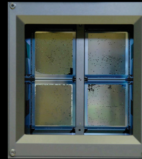
MEMS device – 105x206 micron shutters
