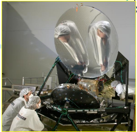
Planck Telescope 1.5x1.9m off-axis Gregorian T = 50 K
