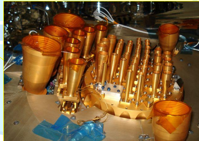
LFI Radiometers 27-77 GHz, T = 20 K
